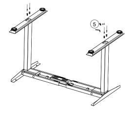
**Step 8-9:** Mount the frame to the table top with 7 5x20 mm wood screws and the handset with 2 5x20 mm wood screws. Tighten the screws.
