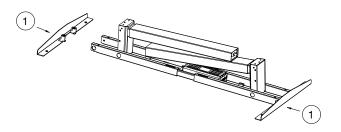
**Step 2-3:** Raise the columns and tighten the screws to the end rail through the frame. Start with the left column followed by the right column.
