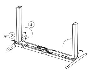
**Step 4:** Ad 8 M6x10 hexagon screw through the frame into the motor house of the columns. Tighten the screws.
