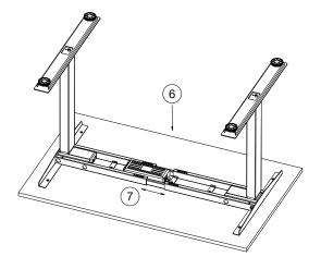
Step 10: Tighten all 8 screws in the frame.
