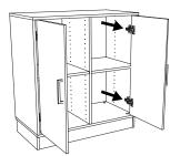
Press the back of the hinges to remove the doors from the cabinet.
