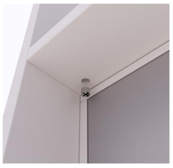
Step 6: Lock all minifixes while still supporting the back plate until the right side is mounted.
