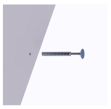
Step 10: Fasten the top plate with screws from above through the pre-drilled holes.
