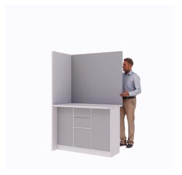
Step 7: Mount the right side and lock all minifixes under the tabletop and in the back plate.
