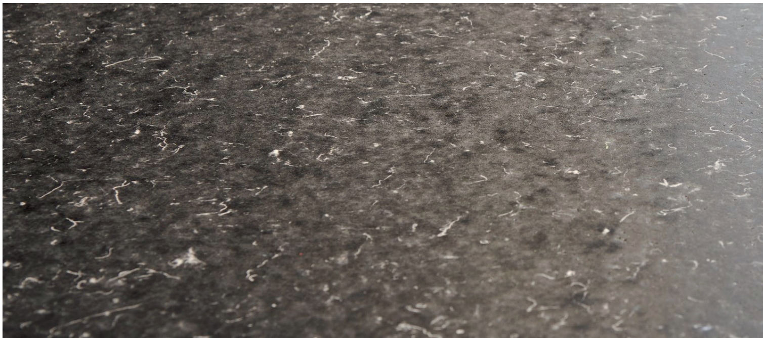
New table top surface: Reznign veneer made of recycled bank suits in black
