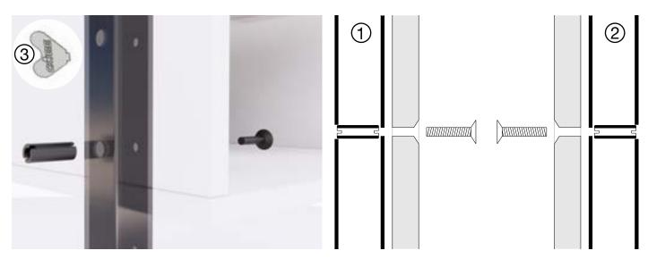
Step 4: Assemble the shelf with the hanger bar using the provided wood screws and shelf brackets.
